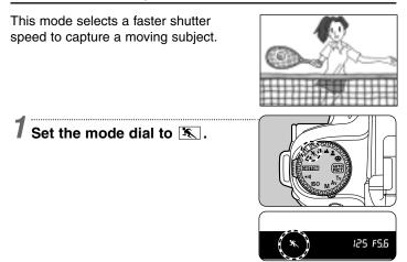
• When the shutter release button is pressed halfway, the shutter speed and aperture setting are displayed in the viewfinder and on the LCD panel. 📧 is also displayed in the viewfinder.
